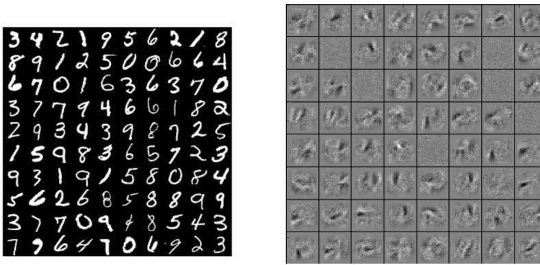
Figure 3: **Left:** Some training examples from the MNIST handwritten digit dataset. Each input is a  $28 \times 28$  grayscale image, which we treat as a 784-dimensional vector. **Right:** A subset of the learned first-layer features. Observe that many of them pick up oriented edges.
